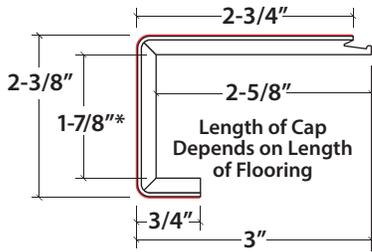
Measure from top of Cap to Stair Riser to cut your planks to the right size
