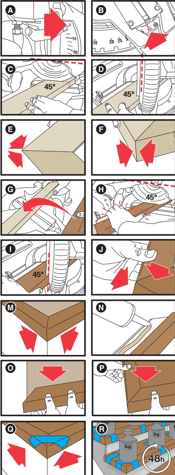
We recommend using a compound miter saw fitted with a **carbide tipped cross blade (60 or 80 teeth, ATB)** for cutting the aluminum VersaEdge Extra Tall molding.
