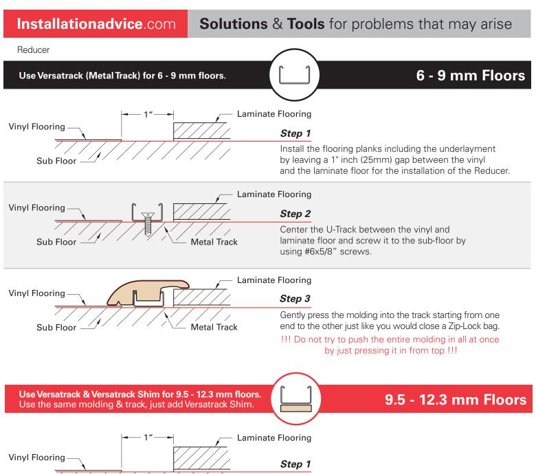
Install the flooring planks including the underlayment by leaving a 1" inch (25mm) gap between the vinyl and the laminate floor for the installation of the Reducer.
